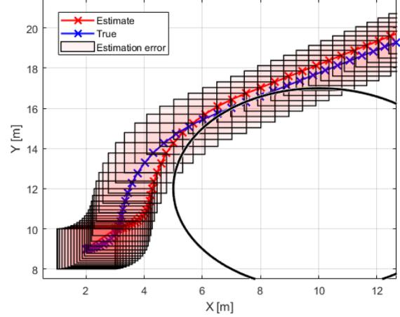
Fig. 1: Simulation using regular high-order CBF under measurement uncertainty. The true trajectory collides with the obstacle (black curve) while the estimate does not.
