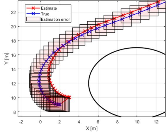
Fig. 2: Simulation using the proposed high-order measurement robust CBF under measurement uncertainty. The true trajectory does not collide with the obstacle.
