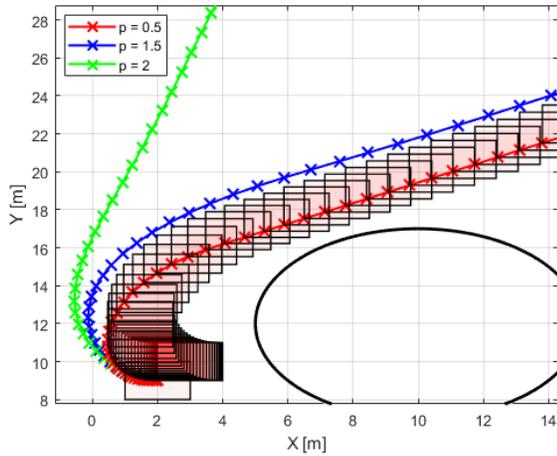
Fig. 3: Simulation using the proposed high-order measurement robust CBF under measurement uncertainty with different penalty values. The conservativeness increases with increasing penalty. The error set is also shown as boxes, for reference.
